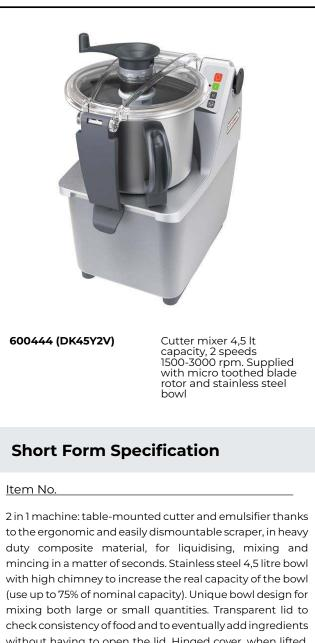
without having to open the lid. Hinged cover, when lifted, remains open to permit a fast and easy check of preparation. Micro toothed blades in 420 AISI stainless steel. All parts are easily dismantled and dishwasher safe. Multiple safety devices ensure the machine will only operate when the cover is properly closed and all parts are correctly positioned. Flat and waterproof control panel with on/off button, pulse function and 2 speeds (1500/3000 rpm).
